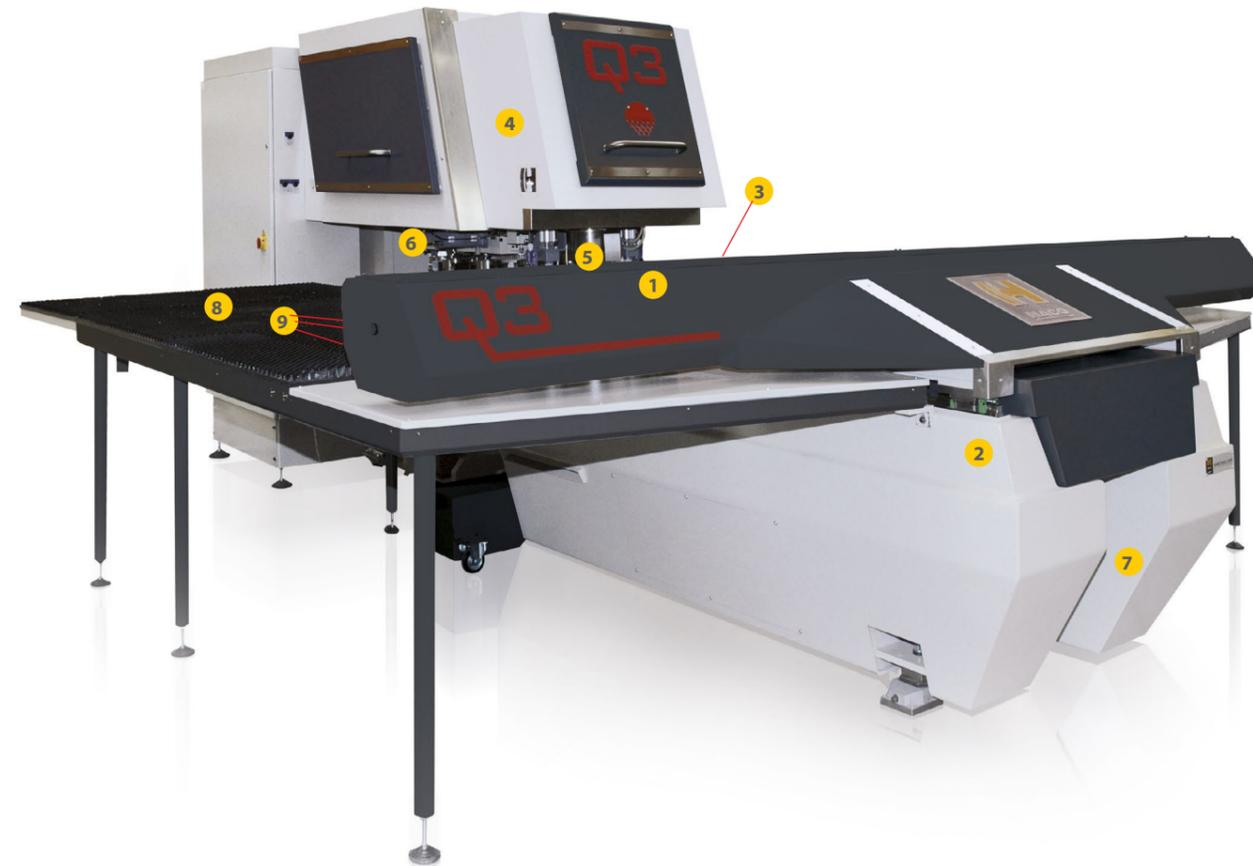
On the large standard brush tables, various workpieces can be nested on standard sheet sizes. The fast AC-servo driven X- and Y-axes with resp. stroke of 2032 by 1524 mm (80" by 60") on Q3 or 2540 by 1524 mm (100" by 60") on Q4 and 3 hydraulic sheet clamps with minimal 'dead zone' 225 by 95 mm ( 8.85" by 3.74") ensure the highest accuracy on all workpieces (optional CNC programmable).
