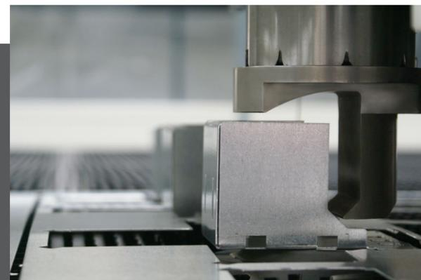
Exceptionally fast forming capabilities. With a bending height of 75mm (3.0 inches) in a variety of angles and even on parts which are nested in other locations than 0° - 45° and 90° your punch press becomes a multifunctional part processing machine.
