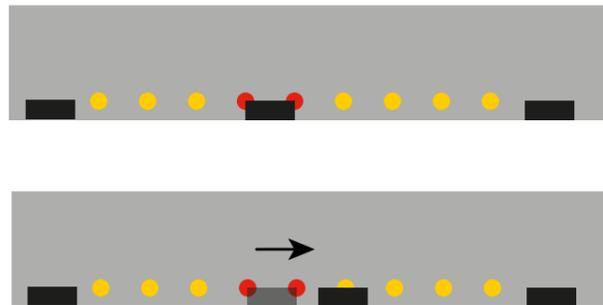
Every clamp is individually movable while the sheet is still clamped by the two other clamps, resulting in better part accuracy. Traditional repositioning with all clamps together can be made as well.
