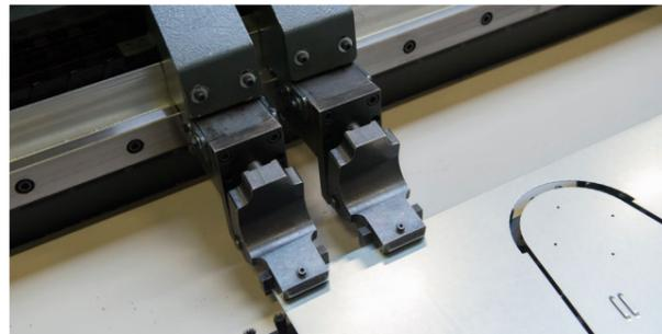
The clamps are set automatically according to the CNC program, minimizing clamp dead zones. When changing production from full size to small sheets, clamp settings can be made automatically without the risk of operator mistakes and without wasting operator time.
