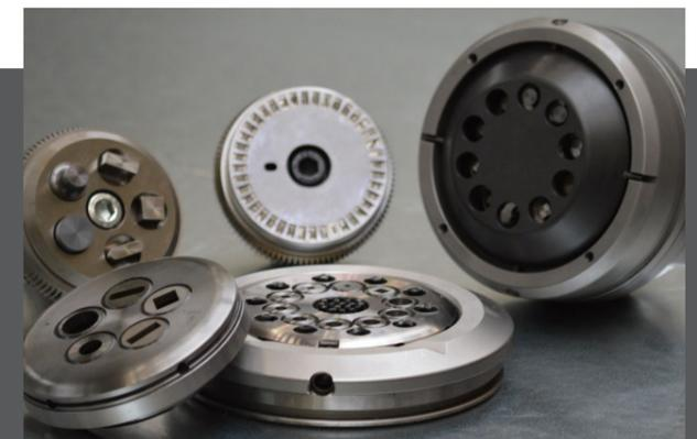
To increase its flexibility even more, the HACO Q-Series can take 5 or 10 station indexable multitools. We offer a complete range of tools for special applications such as louvering, embossing, forming, bending, tapping, 40 character ID stamping, marking and all wheel tools.
