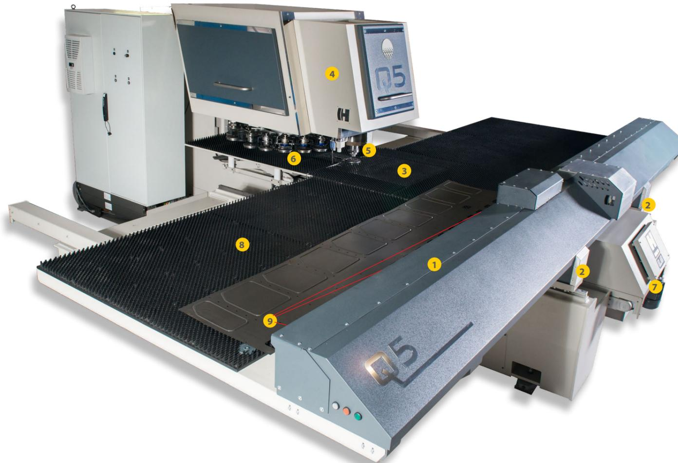
On the large standard brush tables, various workpieces can be nested on standard sheet sizes. The fast AC-servo driven X- and double Y-axes with resp. stroke of 2540 by 1580 mm (100" by 62") or 3000 by 1580 mm (120" by 62") and 3 hydraulic sheet clamps with minimal 'dead zone' 225 by 95 mm ( 8.85" by 3.74") ensure the highest accuracy on all workpieces.
