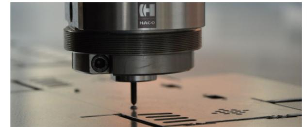
Traditional float tapping or rigid tapping with interpolation, your choice. With the Q series single head punching machines you can use the traditional float tapping system, using a special tap holder. This special float tapping holder will generate the down and up movement for the tap while the C1 axis generating the tap rotation.
